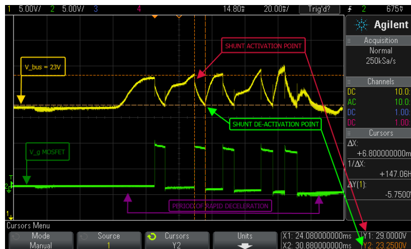
Figure 14: In this application, an Ultra Motion ServoCylinder with a BLDC Motor is rapidly decelerating an 80 lbm mass. The bus voltage (yellow) rapidly rises at the beginning of the period of rapid deceleration until it hits V_{act} = 29V and then quickly drops when the shunt is activated. The shunt activation periods are indicated by high MOSFET voltage (green). The OVP device in the Ultra Motion PSU triggers at 41.6V, and deactivates at 37.5V.
