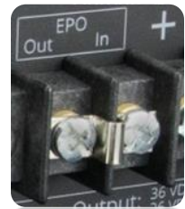
Figure 2: EPO terminals with jumper installed
