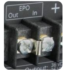
Figure 2: EPO terminals with jumper installed
